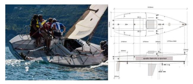
The water lines have been designed to reach the maximum speed in regattas, obtained thanks to the considerable length at the waterline (7.30 metres), performing in tight winds, and to the increasingly flat course of the stern sections, which favor "surfing" at downwind speeds, especially with formed waves. The stability of shape allows to easily keep the boat in its water lines, despite the natural tendency to heel due to cross winds.
